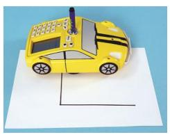
**Pen Mechanism** Pro-Bot has a pen mechanism which holds a standard felt-tip pen enabling Pro-Bot to draw as it moves. This allows Pro-Bot to leave a written record of its route as it moves which makes it easy to analyze the program and decide on changes and refinements. The pen mechanism also allows Pro-Bot to be used as a drawing mechanism to make interesting shapes and pictures.
